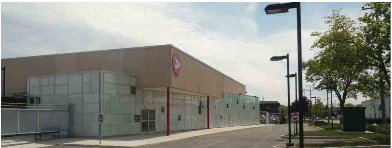
Material changes and vertical articulation along the façade of this building minimize the visual perception of the relatively long façade.
